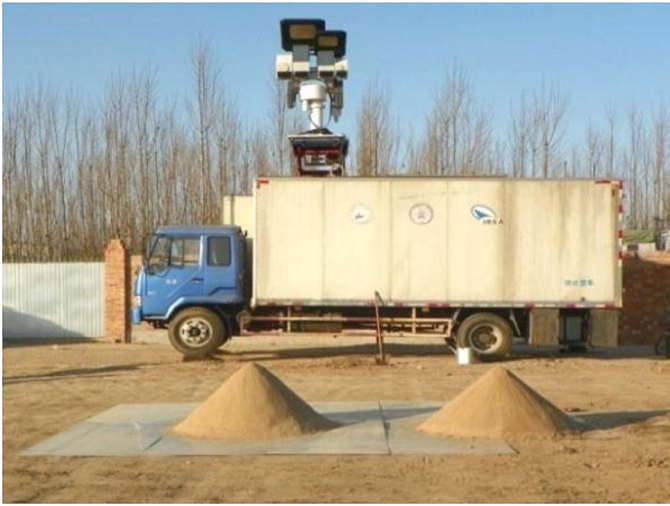
Fig. 1. Two constructed conical hills perpendicular to the radiometer (slope angle of 40^\circ ) within the 4 \text{ m}^2 footprint of the TMMR. The visible footprint for TMMR is 1.5 \times 1.5 \text{ m} covered by one hill (left), and the other hill (right) stands out of the view to observe the adjacent effect on the visual field.
